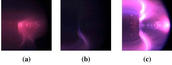
Figure 1. Images of plasma shape captured with a camera on the HL-3 device. (a) Displays the inner limiter shape in shot #06696, with window interference present on the wall. (b) Is the divertor shape related to shot #06696, wherein the image exhibits low brightness levels, leading to a loss of edge recognition. (c) Is a gas puffing interference image in shot #06255, with bright air delivery interference spots visible on the wall.
